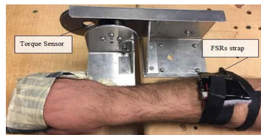
Figure 2: The setup for collecting flexion-extension data.
