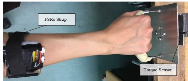
Figure 1: The setup for collecting pronation - supination data.
